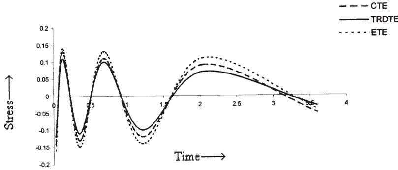
Figure 1: Distribution of normal stress  $\tau_{11}$  (for  $y = 1, z = 1,$  and  $\Omega = 10^5$ ) versus time
