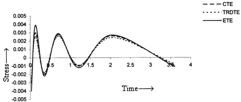
Figure 4: Distribution of normal stress  $\tau_{23}$  (for  $y = 1$ ,  $z = 1$ , and  $\Omega = 10^5$ ) versus time
