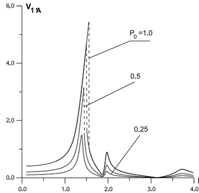
Figure 3: Amplitude-frequency curves for  $V_1$  in a hard characteristic case
