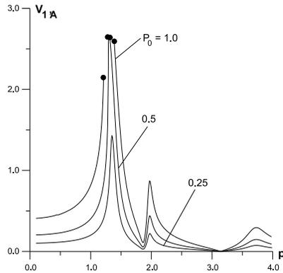
Figure 2: Amplitude-frequency curves for  $V_1$  in a soft characteristic case
