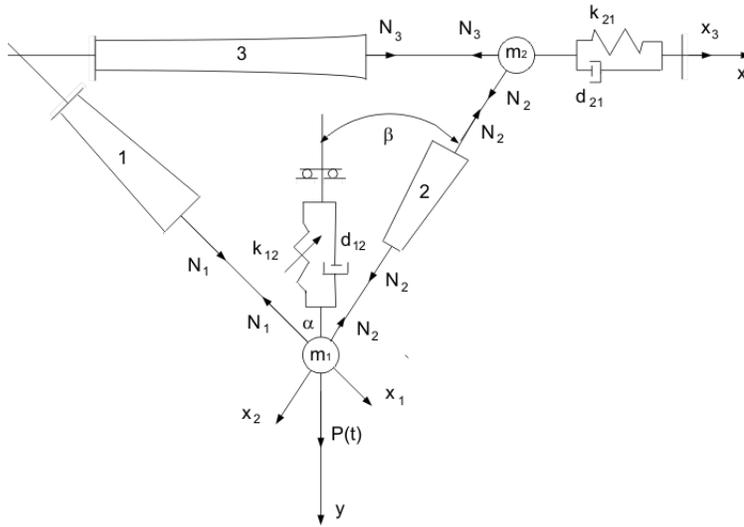
Figure 1: Two-mass rod system
