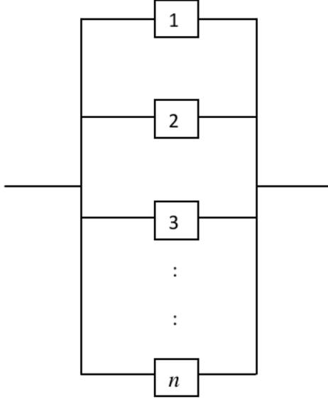
Figure 4: System 4 ( $n$ -component parallel system)
