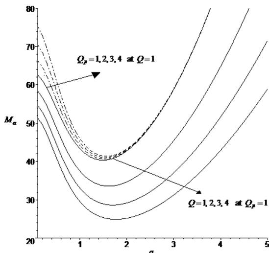
Figure 3: Critical Marangoni number  $M_{ac}$  at the onset of convection as a function of wavenumber,  $a$  for a ranges of values of  $Q$  and  $Q_p$  in the case  $\alpha = 0.1$ ,  $\zeta = 1$  and  $Da = 0.003$
