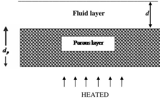
Figure 1: The saturated porous layer heated from below
