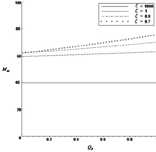
Figure 5: Critical Marangoni number  $M_{ac}$  at the onset of convection as a function of  $Q_p$  for a ranges of values of  $\zeta$  in the case  $\alpha = 0.1$ ,  $Q = 1$  and  $Da = 0.003$
