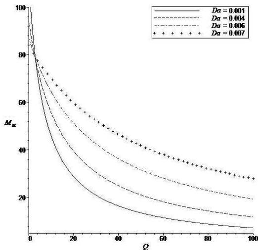
Figure 6: Critical Marangoni number  $M_{ac}$  at the onset of convection as a function of  $Q$  for a ranges of values of  $Da$  in the case  $Q_p = 1$
