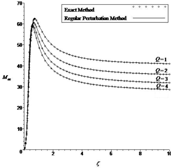
Figure 2: Critical Marangoni number  $M_{ac}$  at the onset of convection as a function of  $\zeta$  in the case  $Q_p = 0$  and  $Da = 0.003$
