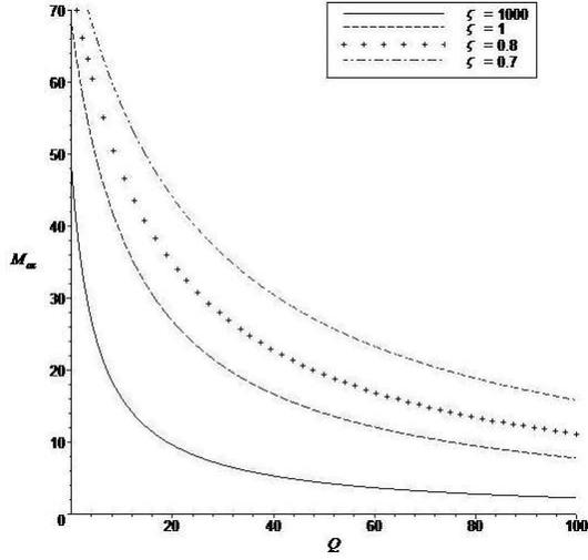
Figure 4: Critical Marangoni number  $M_{ac}$  at the onset of convection as a function of  $Q$  for a ranges of values of  $\zeta$  in the case  $\alpha = 0.1$ ,  $Q_p = 1$  and  $Da = 0.003$
