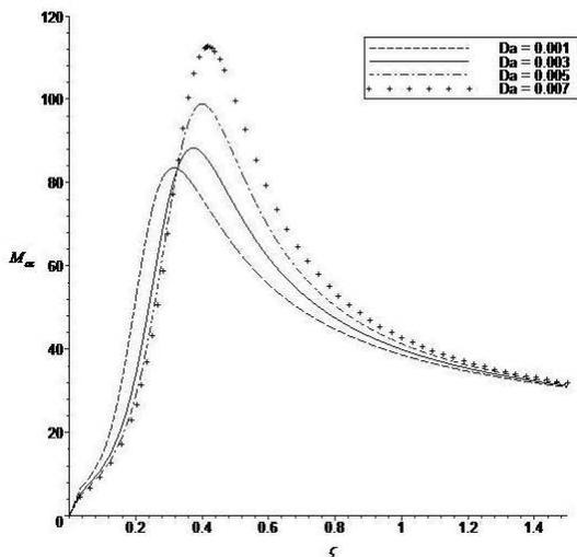
Figure 7: Critical Marangoni number  $M_{ac}$  at the onset of convection as a function of  $\zeta$  for a ranges of values of  $Da$  in the case  $Q = 10$  and  $Q_p = 0$
