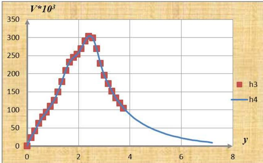
Figure 5: Graph show the horizontal velocity distribution along the  $Oy$  axis,  $v(y)$  at the time moment  $t = 6$  for Reynolds number  $Re = 310^5$  in the center of spot. Solid line denotes data, obtained on scheme, considered in current paper, rectangular – data, obtained on scheme of third order accuracy [8].
