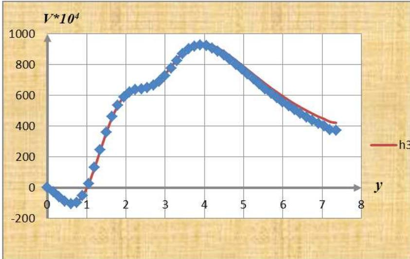
Figure 4: Graph show the horizontal velocity distribution along the Oy axis,  $v(y)$  at the time moment  $t = 12$  for Reynolds number  $Re = 300$  in the center of spot. Solid line denotes data, obtained on scheme of third order accuracy [8], rectangular – data, obtained on scheme, considered in current paper.
