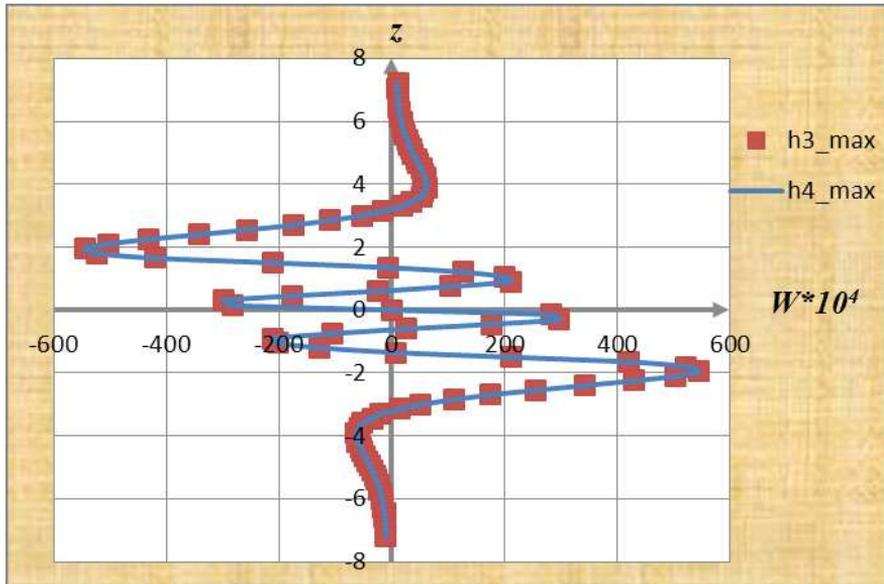
Figure 13: Graph show the vertical velocity distribution along the  $Oz$  axis,  $w(z)$  at the time moment  $t = 12$  for Reynolds number  $Re = 310^5$  in the region of amplitudes. Solid line denotes data, obtained on scheme, considered in current paper, rectangular – data, obtained on scheme of third order accuracy [8].
