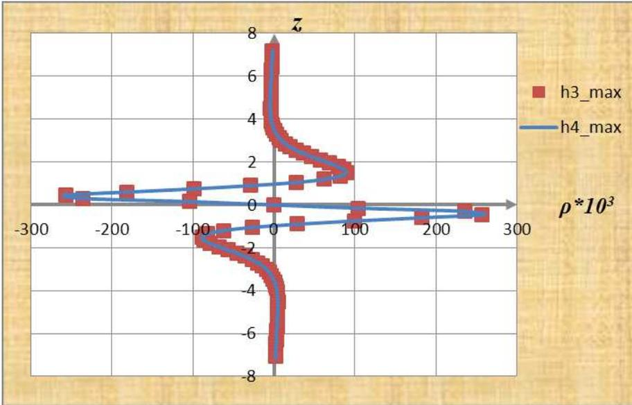
Figure 19: Graph show the density distribution along the Oz axis,  $\rho(z)$  at the time moment  $t = 6$  for Reynolds number  $Re = 310^5$  in the region of maximum amplitudes. Solid line denotes data, obtained on scheme, considered in current paper, rectangular – data, obtained on scheme of third order accuracy [8].
