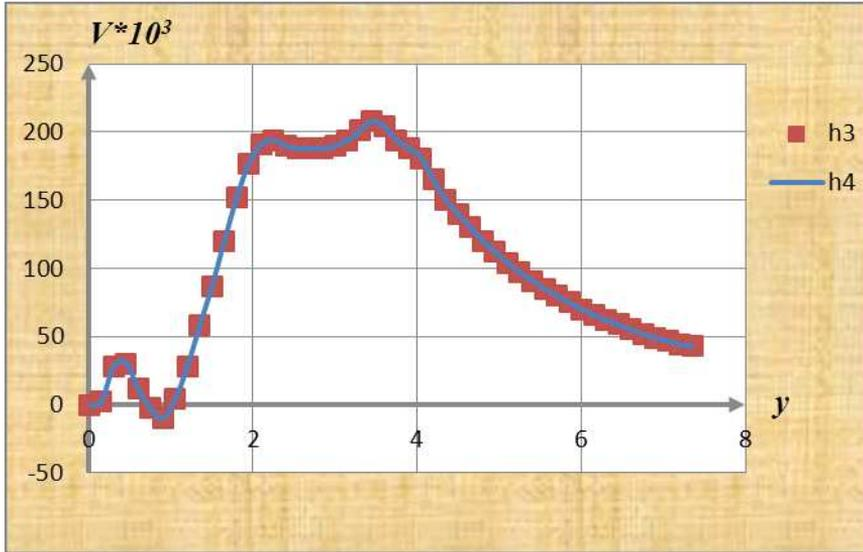
Figure 6: Graph show the horizontal velocity distribution along the  $Oy$  axis,  $v(y)$  at the time moment  $t = 12$  for Reynolds number  $Re = 310^5$  in the center of spot. Solid line denotes data, obtained on scheme, considered in current paper, rectangular – data, obtained on scheme of third order accuracy [8].
