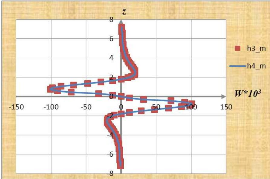
Figure 12: Graph show the vertical velocity distribution along the Oz axis,  $w(z)$  at the time moment  $t = 6$  for Reynolds number  $Re = 310^5$  in the region of amplitudes. Solid line denotes data, obtained on scheme, considered in current paper, rectangular – data, obtained on scheme of third order accuracy [8].
