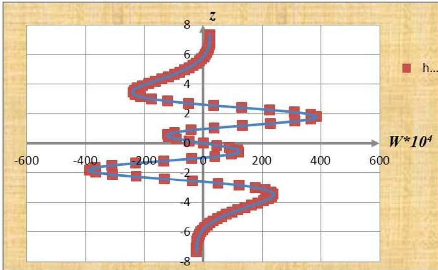
Figure 11: Graph show the vertical velocity distribution along the Oz axis,  $w(z)$  at the time moment  $t = 12$  for Reynolds number  $Re = 310^2$  in the region of amplitudes. Solid line denotes data, obtained on scheme, considered in current paper, rectangular – data, obtained on scheme of third order accuracy [8].
