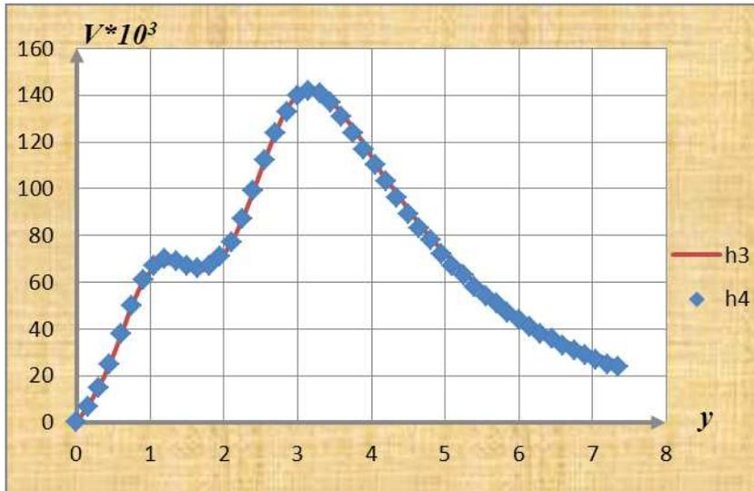
Figure 3: Graph show the horizontal velocity distribution along the Oy axis,  $v(y)$  at the time moment  $t = 9$  for Reynolds number  $Re = 300$  in the center of spot. Solid line denotes data, obtained on scheme of third order accuracy [8], rectangular – data, obtained on scheme, considered in current paper.
