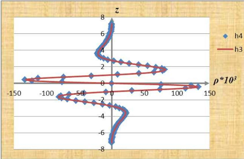
Figure 17: Graph show the density distribution along the Oz axis,  $\rho(z)$  at the time moment  $t = 9$  for Reynolds number  $Re = 310^2$  in the region of maximum amplitudes. Solid line denotes data, obtained on scheme of third order accuracy [8], rectangular – data, obtained on scheme considered in current paper.
