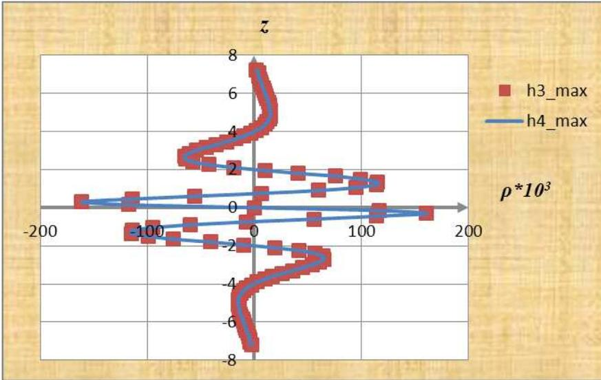
Figure 20: Graph show the density distribution along the  $Oz$  axis,  $\rho(z)$  at the time moment  $t = 12$  for Reynolds number  $Re = 310^5$  in the region of maximum amplitudes. Solid line denotes data, obtained on scheme, considered in current paper, rectangular – data, obtained on scheme of third order accuracy [8].
