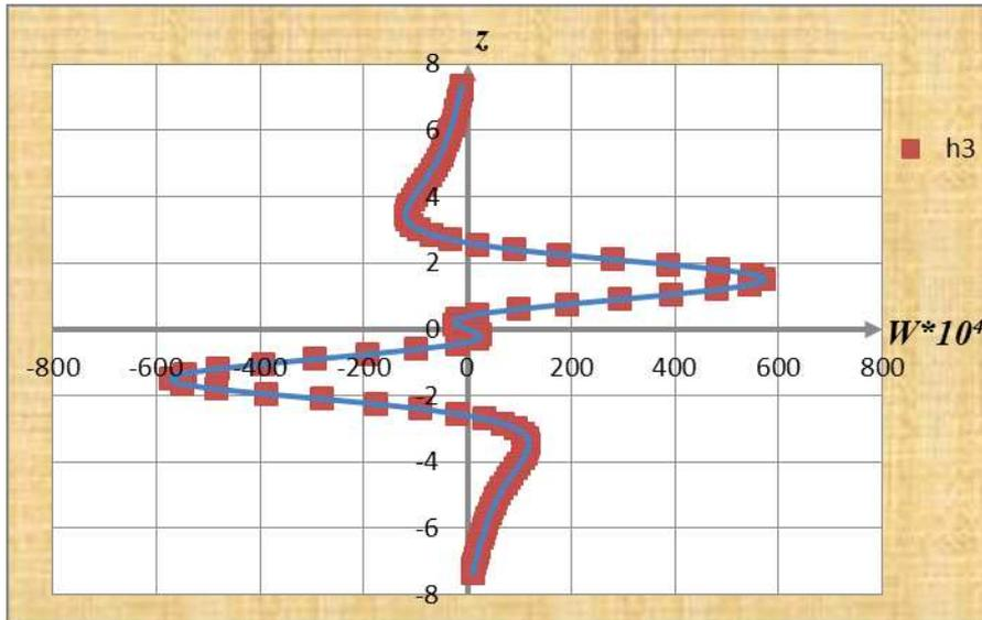
Figure 9: Graph show the vertical velocity distribution along the Oz axis,  $w(z)$  at the time moment  $t = 9$  for Reynolds number  $Re = 310^2$  in the region of maximum amplitudes. Solid line denotes data, obtained on scheme, considered in current paper, rectangular – data, obtained on scheme of third order accuracy [8].
