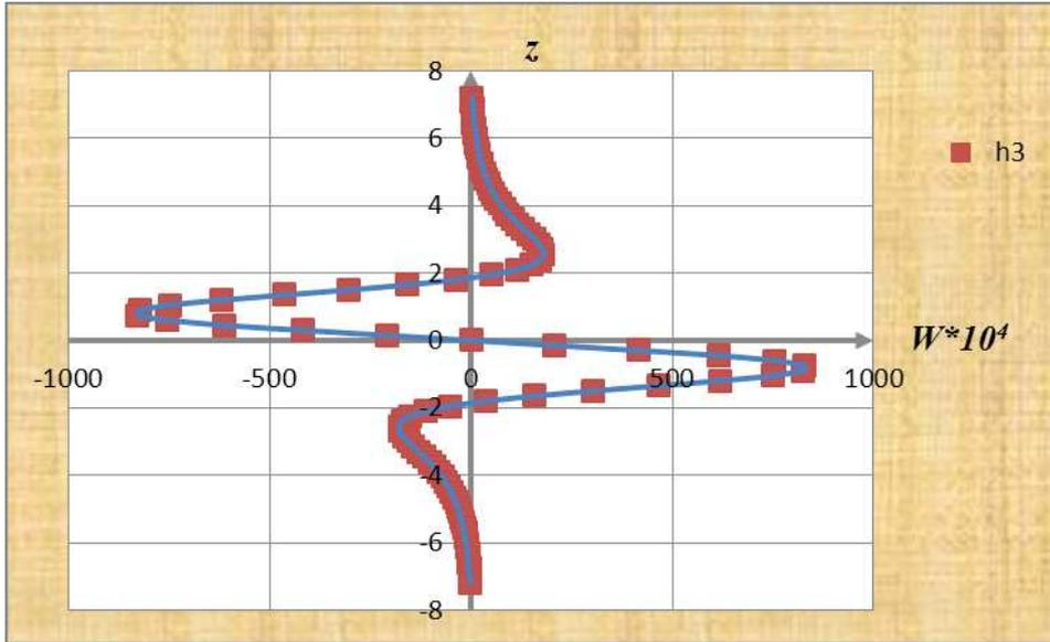
Figure 8: Graph show the vertical velocity distribution along the  $Oz$  axis,  $w(z)$  at the time moment  $t = 6$  for Reynolds number  $Re = 310^2$  in the region of maximum amplitudes. Solid line denotes data, obtained on scheme, considered in current paper, rectangular – data, obtained on scheme of third order accuracy [8].
