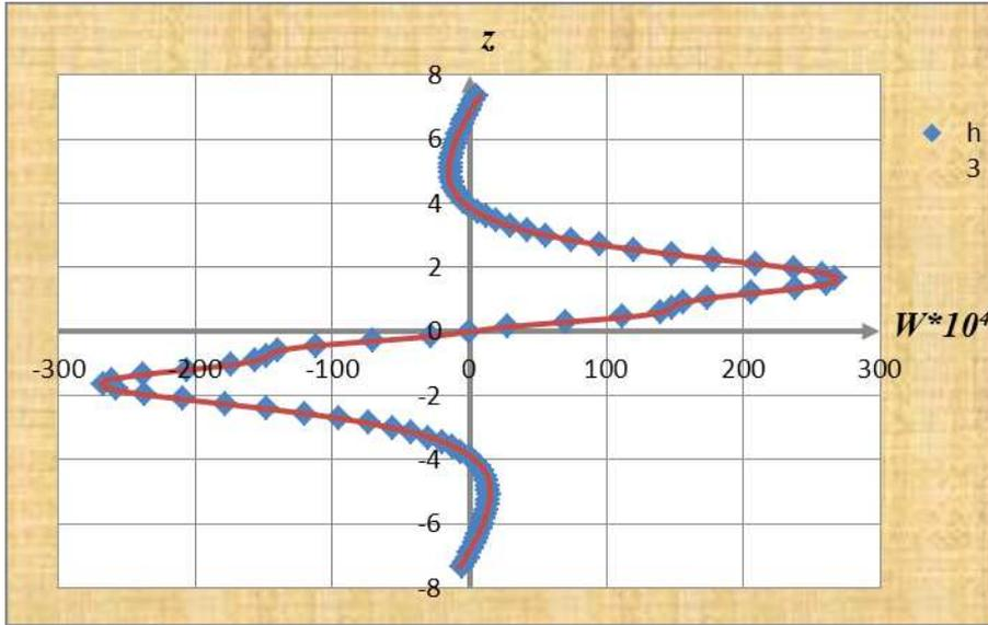
Figure 10: Graph show the vertical velocity distribution along the  $Oz$  axis,  $w(z)$  at the time moment  $t = 12$  for Reynolds number  $Re = 310^2$  in the center of spot. Solid line denotes data, obtained on scheme, considered in current paper, rectangular – data, obtained on scheme of third order accuracy [8].
