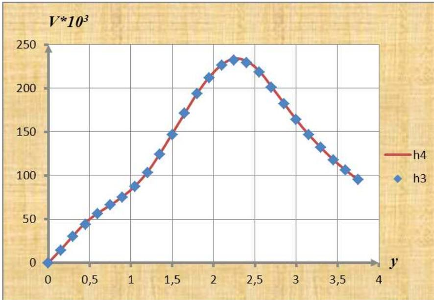
Figure 2: Graph show the horizontal velocity distribution along the  $Oy$  axis,  $v(y)$  at the time moment  $t = 6$  for Reynolds number  $Re = 300$  in the center of spot. Solid line denotes data, obtained on scheme, considered in current paper, rectangular – data, obtained on scheme of third order accuracy [8].
