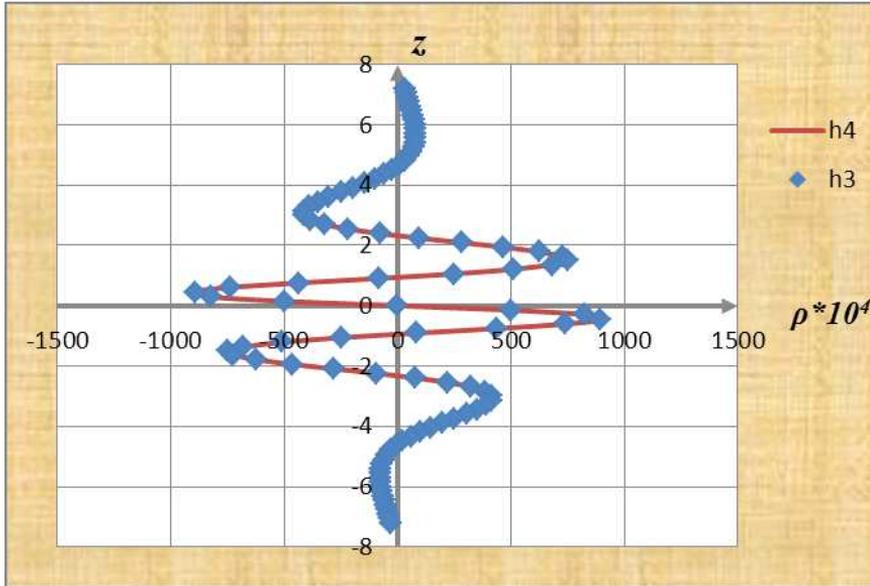
Figure 18: Graph show the density distribution along the Oz axis,  $\rho(z)$  at the time moment  $t = 12$  for Reynolds number  $Re = 310^2$  in the region of maximum amplitudes. Solid line denotes data, obtained on scheme, considered in current paper, rectangular – data, obtained on scheme of third order accuracy [8].
