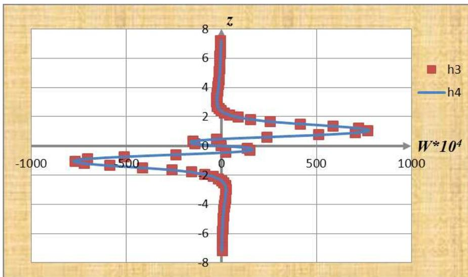
Figure 7: Graph show the vertical velocity distribution along the Oz axis,  $w(z)$  at the time moment  $t = 6$  for Reynolds number  $Re = 310^2$  in the center of spot. Solid line denotes data, obtained on scheme, considered in current paper, rectangular – data, obtained on scheme of third order accuracy [8].
