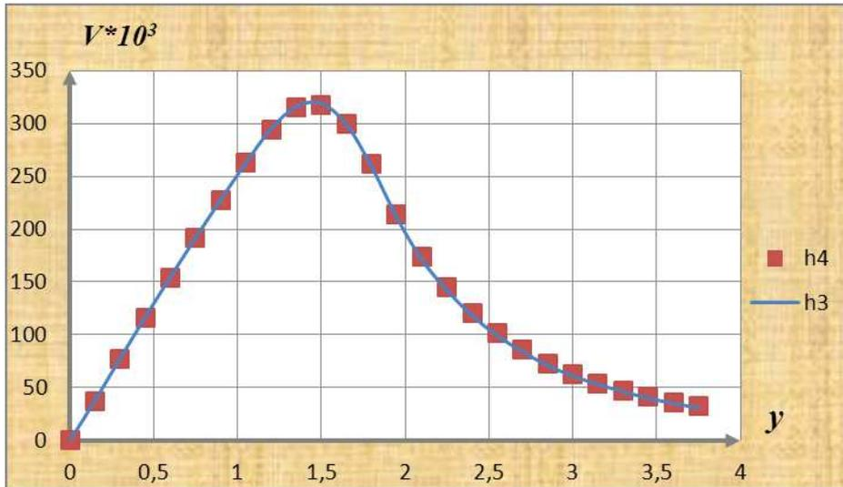
Figure 1: Graph show the horizontal velocity distribution along the Oy axis,  $v(y)$  at the time moment  $t = 3$  for Reynolds number  $Re = 300$  in the center of spot. Solid line denotes data, obtained on scheme of third order accuracy [8], rectangular – data, obtained on scheme, considered in current paper.
