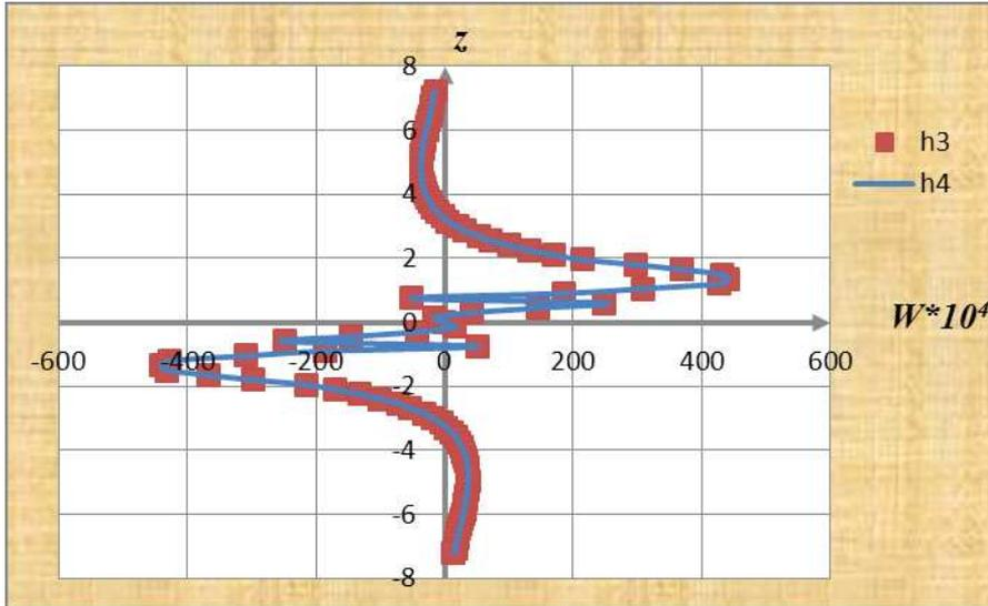
Figure 14: Graph show the vertical velocity distribution along the Oz axis,  $w(z)$  at the time moment  $t = 12$  for Reynolds number  $Re = 310^5$  in the center of Solid line denotes data, obtained on scheme, considered in current paper, rectangular – data, obtained on scheme of third order accuracy [8].
