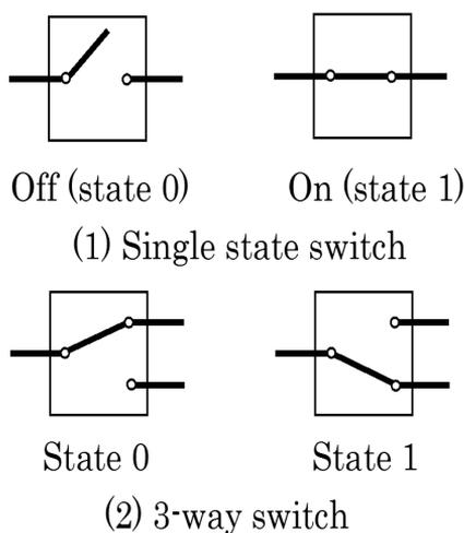
Figure 3: Single state switch and 3-way switch
