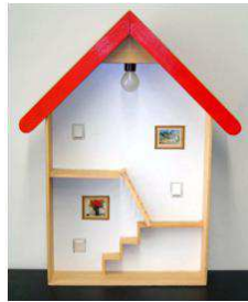
Figure 5: Stairway switches on three floors
