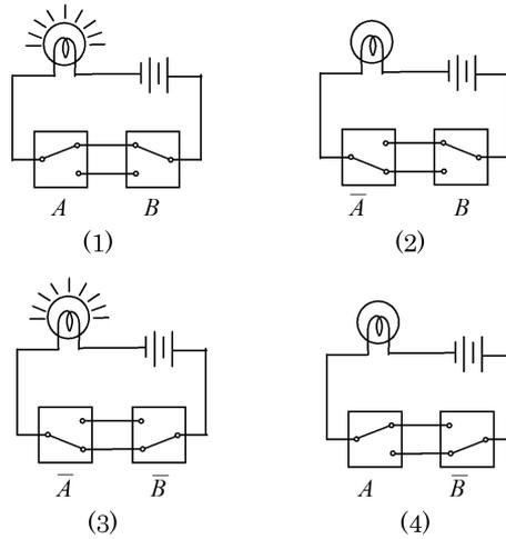
Figure 4: Switches in two places (set of four)
