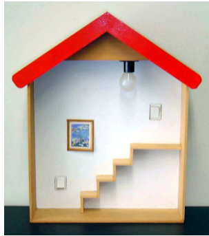
Figure 1: Stairway switches on two different floors
