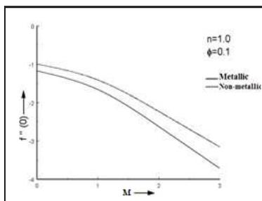
Figure 4: Effects of parameter  $M$  on skin friction coefficient for different types of nanoparticles
