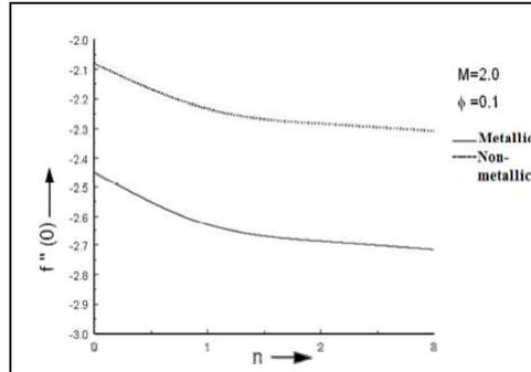
Figure 5: Effects of parameter  $n$  on skin friction coefficient for different types of nanoparticles
