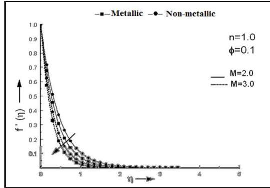
Figure 1: Effects of  $M$  on velocity profile  $f'(\eta)$  for different types of nanoparticles
