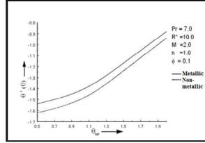
Figure 7: Effects of surface temperature parameter  $\theta_w$  on heat transfer rate for different types of nanoparticles
