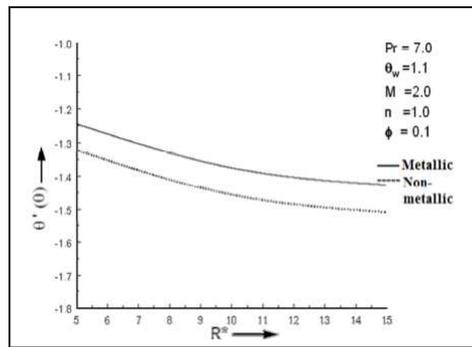
Figure 6: Effects of thermal radiation parameter  $R^*$  on heat transfer rate for different types of nanoparticles
