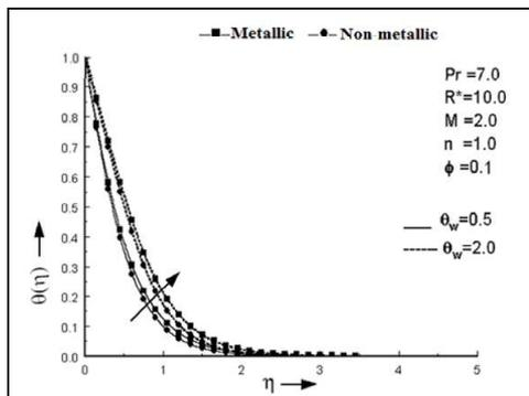
Figure 3: Effects of surface temperature parameter  $\theta_w$  on the temperature profile  $\theta(\eta)$  for different types of nanoparticles
