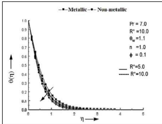
Figure 2: Effects of thermal radiation parameter  $R^*$  on temperature profile  $\theta(\eta)$  for different types of nanoparticles
